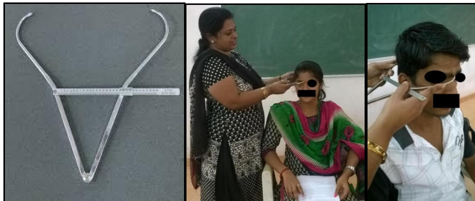
Fig 4- Spreading caliper with rounded ends, Researcher taking Head length measurement
