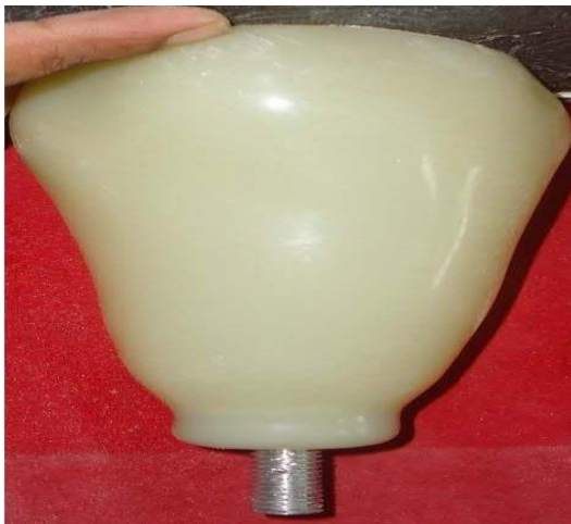
Fig 4. Polyethylene moulded socket with 12mm rod
